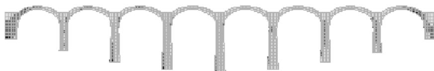
Figure 10 : Failure results due to  $\sigma_1^D, \sigma_3^D$
