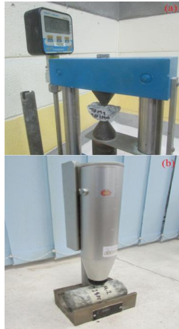
Fig. 3 Conducted tests of (a) point load strength and (b) Schmidt hammer
