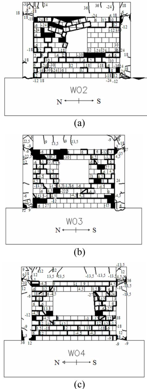
Figure 7. Failure modes of specimens with window openings.
