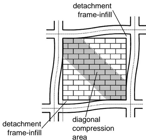
Figure 1. Strut model analogy of in-filled frames.
