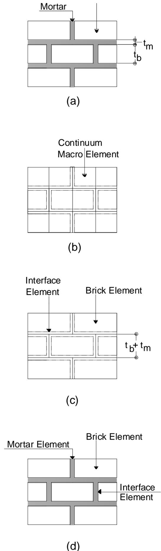
Figure 3: Masonry modeling strategies: a) Masonry sample; b) Macro-modeling; c) Simplified micro-modeling; d) Detailed micro-modeling
