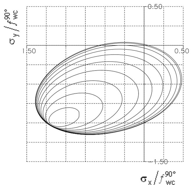
Figure 2: Non-Dimensional Failure Surface of Masonry in Normal Stress Terms (Asteris et al., 2009) ( $\tau/f_{wc}^{90^\circ} = 0.00$  up to  $0.45$  by step= $0.05$ )
