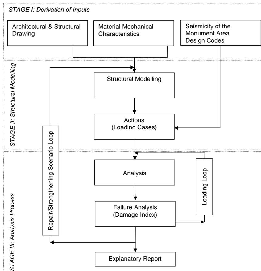
Figure 1: Flowchart with the applied methodology for vulnerability and restoration assessment
