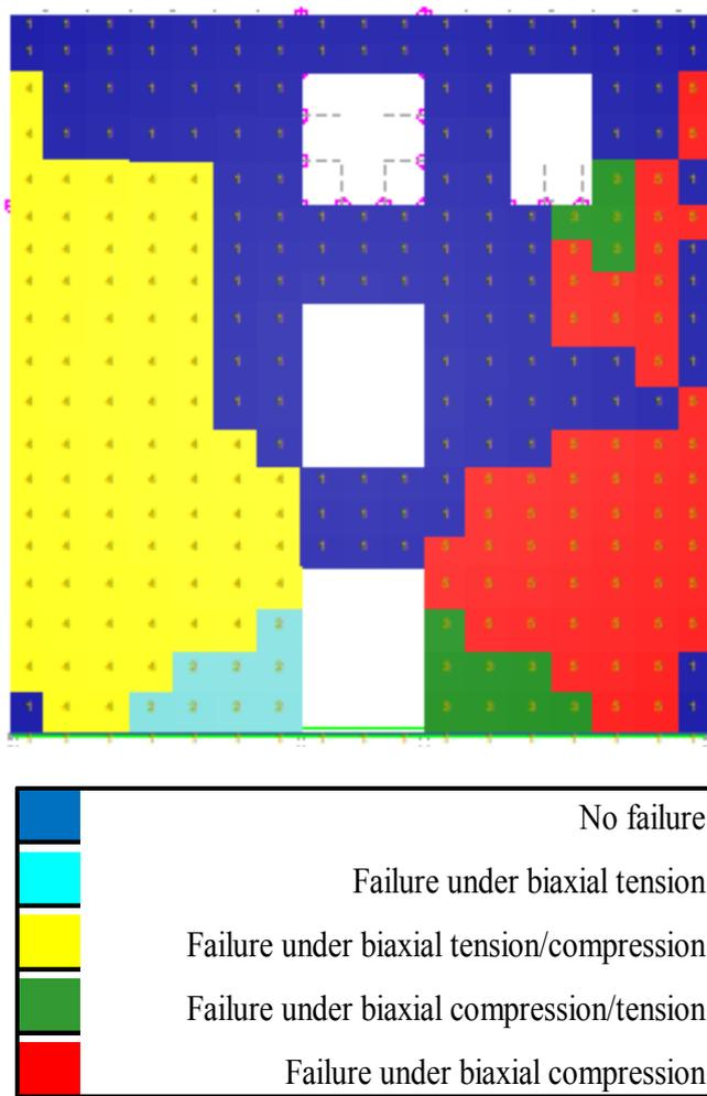
Figure 7: Illustration of failed elements and type of failure for a typical masonry wall before interventions (Wall 6)
