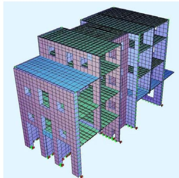
Figure 5: The 3-D FEM model of the building
