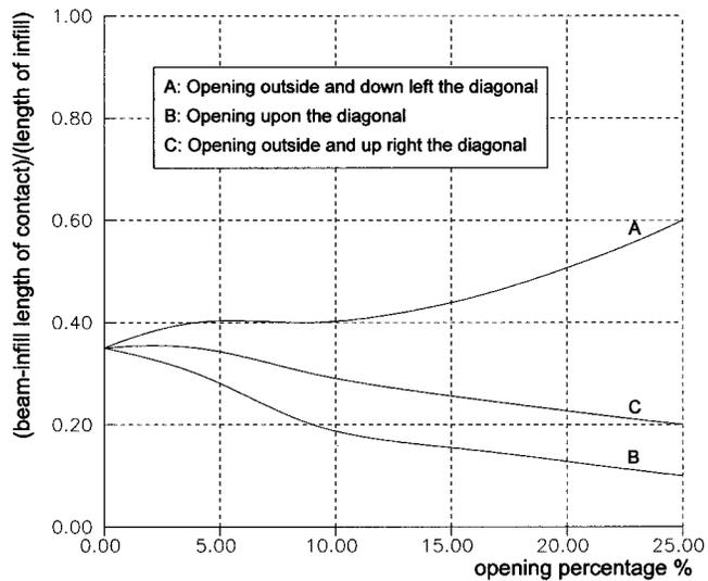
Fig. 7. Beam/infill length of contact as function of opening percentage
