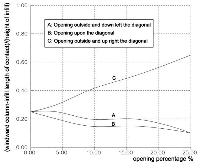
Fig. 8. Windward column/infill length of contact as function of opening percentage
