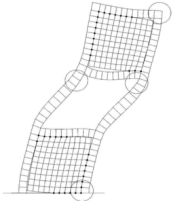
**Fig. 13.** Deformed mesh and main areas of higher vulnerability in three-story one-bay infilled frame with soft second story
