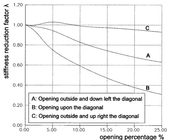
**Fig. 5.** Stiffness reduction factor  $\lambda$  of infilled frame in relation to opening percentage for different positions of opening
