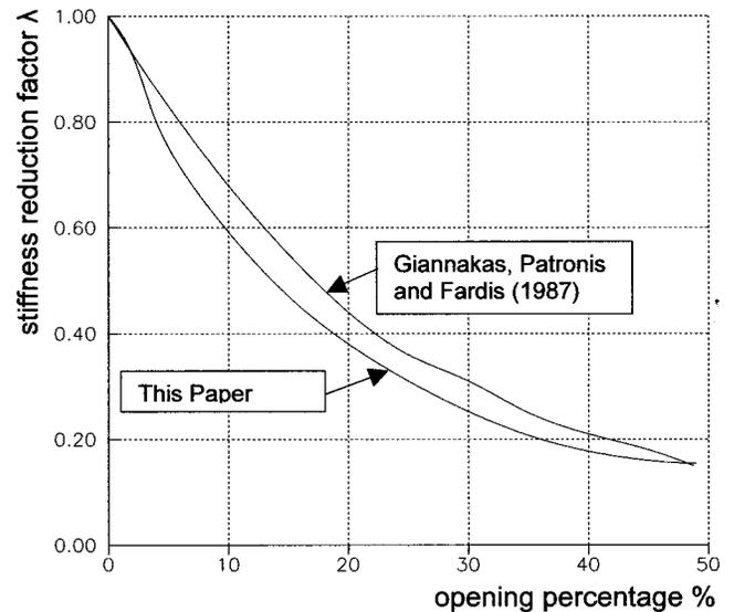
**Fig. 4.** Stiffness reduction factor  $\lambda$  of infilled frame in relation to opening percentage (case B: opening upon compressed diagonal)
