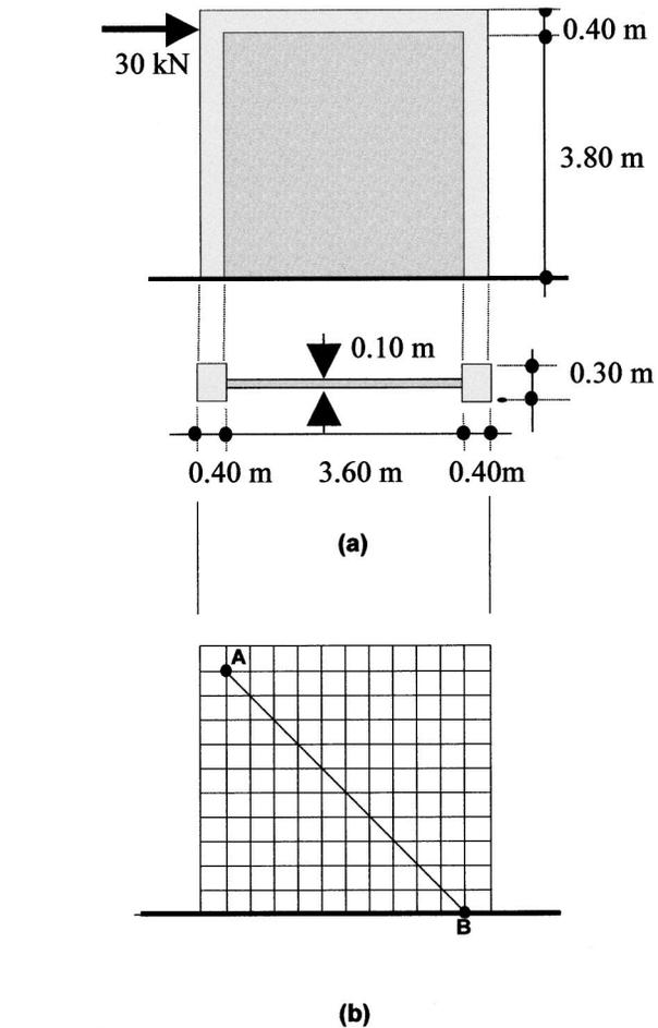
Fig. 1. One-story one-bay brickwork infilled frame: (a) geometry and loading; (b) mesh
