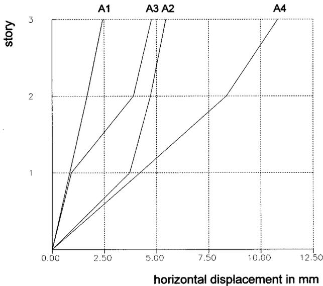
**Fig. 9.** Story displacements for different arrangements of infill wall
