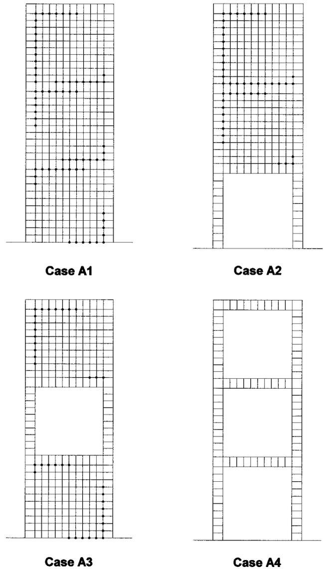
**Fig. 10.** Contact areas between surrounding frame and infill walls for four different cases of infill wall arrangement
