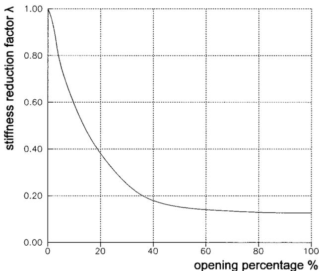
**Fig. 3.** Stiffness reduction factor  $\lambda$  of infilled frame in relation to opening percentage (case B: opening upon compressed diagonal)
