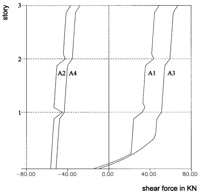
**Fig. 12.** Shear force diagram for right column of three-story one-bay infilled frame (see Fig. 10). Positive shear force indicates clockwise shear force
