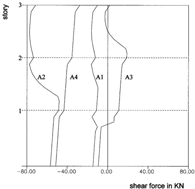
**Fig. 11.** Shear force diagram for windward column of three-story one-bay infilled frame (see Fig. 10). Positive shear force indicates clockwise shear force
