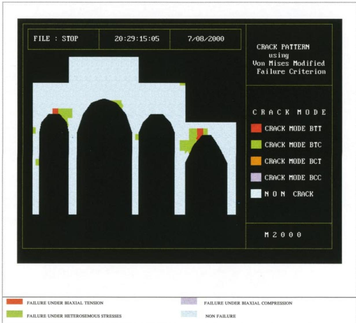
Fig. 5. (Color) Failure results of internal wall, before interventions
