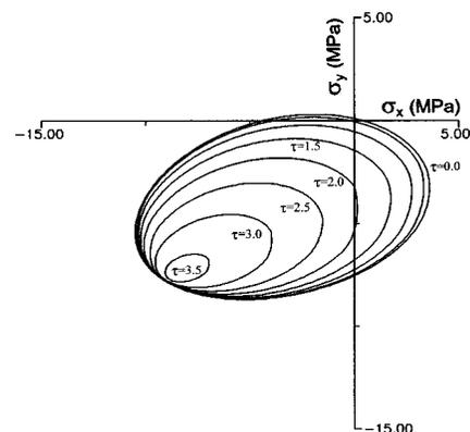
Fig. 4. Failure surface of masonry in normal stress terms
