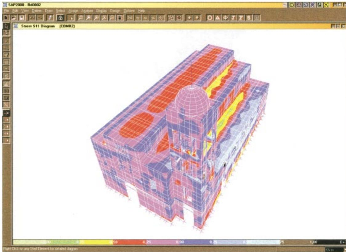
Fig. 3. (Color) Typical graphical output of the analysis results before interventions (biaxial stress  $\sigma_{xx}$ —loading case 2)
