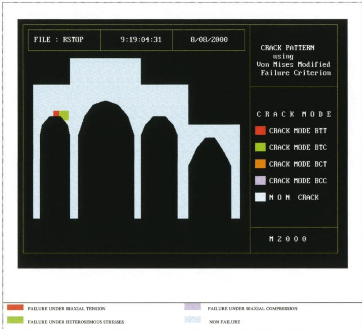
Fig. 6. (Color) failure results of internal wall, after interventions
