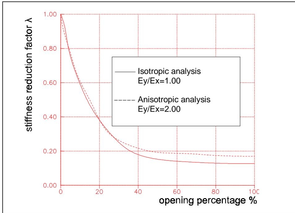
Figure 5. Stiffness reduction factor  $\lambda$  of the infilled frame in relation to the opening percentage for isotropic and anisotropic analysis
