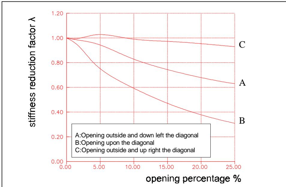
Figure 3. Stiffness reduction factor  $\lambda$  of the infilled frame in relation to the opening percentage
