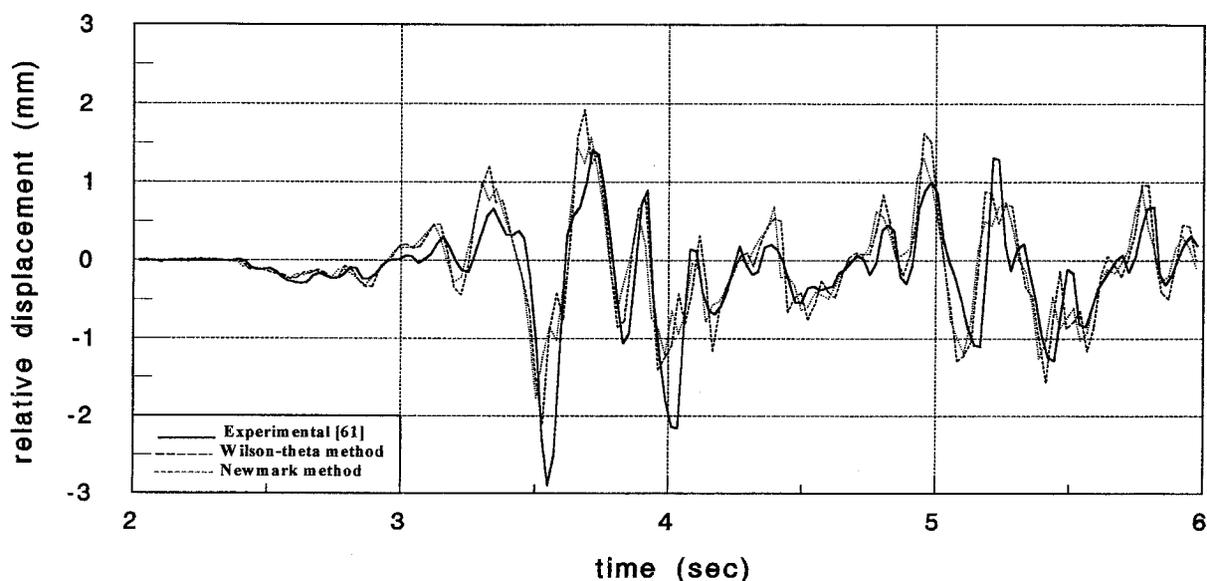
Fig. 6. Comparison of the computed seismic responses of the wall of Fig. (4) to the excitation of Fig. (5)
