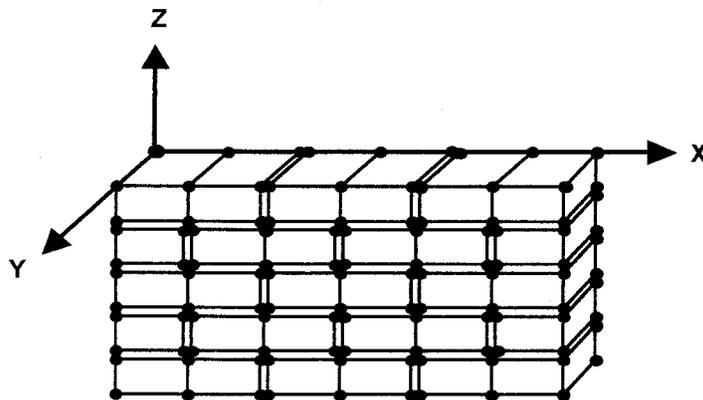
Fig. 2. Typical finite element subdivision
