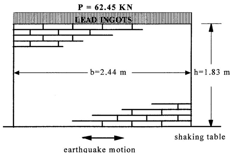
Fig. 4. Schematic diagram of the seismic test setup
