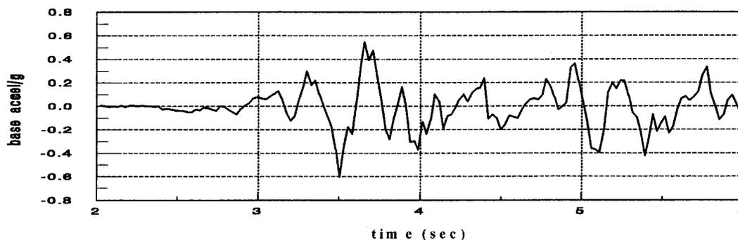
Fig. (5). Seismic record of the modified El Centro earthquake (taken from [Mengi 1986])
