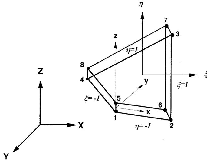
Fig. 1. Geometry of the 3-D interface element
